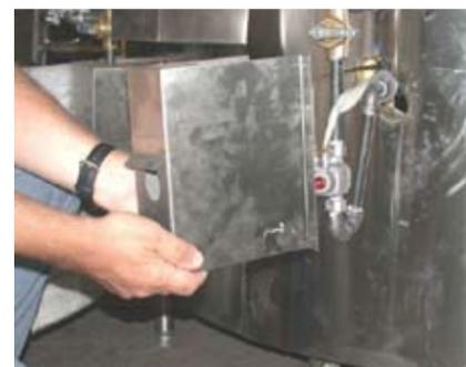
1. Remove the valve/control cover
