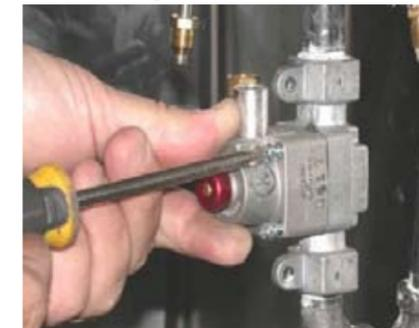
4. Remove the screws from the safety head.
