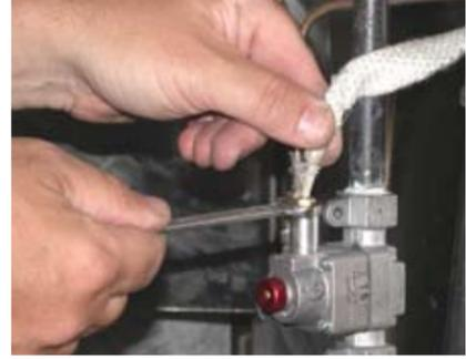
12. Thread the thermocouple fitting into the body by hand. When you can no longer tighten by hand, use a 3/8" wrench to make snug. A good rule is giving a 1/8 turn after finger tightening. **DO NOT OVERTIGHTEN** as it will damage the control. Turn on gas, check for leaks, and relight pilot.
