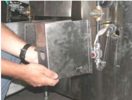
1. Remove the valve/control cover
